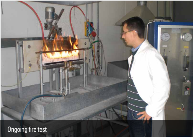
Flame and mechanical shock BS 50200
